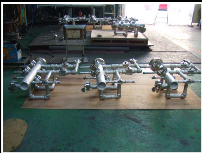
운활유 LINE PIGGING SYSTEM
